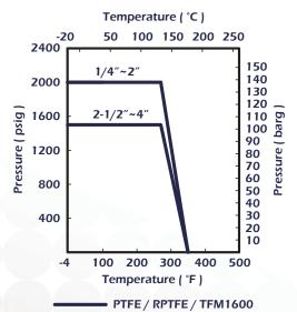
This table express Seat material resistance as declared by the original manufacturers. The values are to be considered with other parameters such as size, seat design and temperature limitations as governed by relevant standards such as ASME B16.34 or EN-12516.
